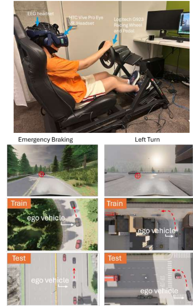
Figure 2. Upper: The dataset collection environment. The HTC VIVE Pro Eye VR headset and Logitech G923 Racing Wheel and Pedal give the subject a more realistic driving experience. Lower: the example of scene image of driver’s view, camera’s view, and bird’s eye view.
